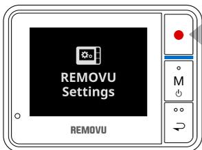
The settings can be adjusted in the Setting Mode. Please navigate to the settings mode using the M (Mode / Power) button, and enter the menu by pressing the REC (Shutter / Select) button
