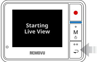
Press and hold the Back button for about 2 seconds to turn on the GoPro. The Live view will be displayed soon after the Starting Live View message appears.
