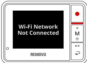
1. Flashing red LED and Wi-Fi Network Not Connected message will appear if Wi-Fi fails to connect or lose its signal.
