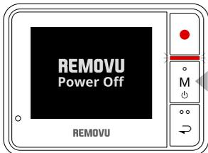
1. Press the M (Mode / Power) button for about 2 seconds to turn off the device. REMOVU Power off logo will appear then the device will be turned off with the red LED blinking three times.
