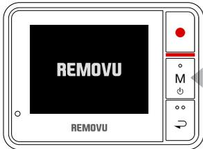
1. Press the M (Mode / Power) button for about 1 second to turn on the power.
