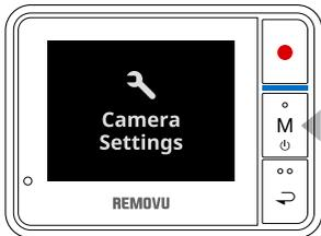
The camera settings can be adjusted in the Setting Mode. Please navigate to the Settings mode by pressing M (Mode / Power) button repeatedly until above screen appears.
