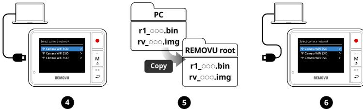
4. When “Select Camera Network” list appears on the REMOVU screen, connect the device to your PC or Mac using the USB cable included in the package.
